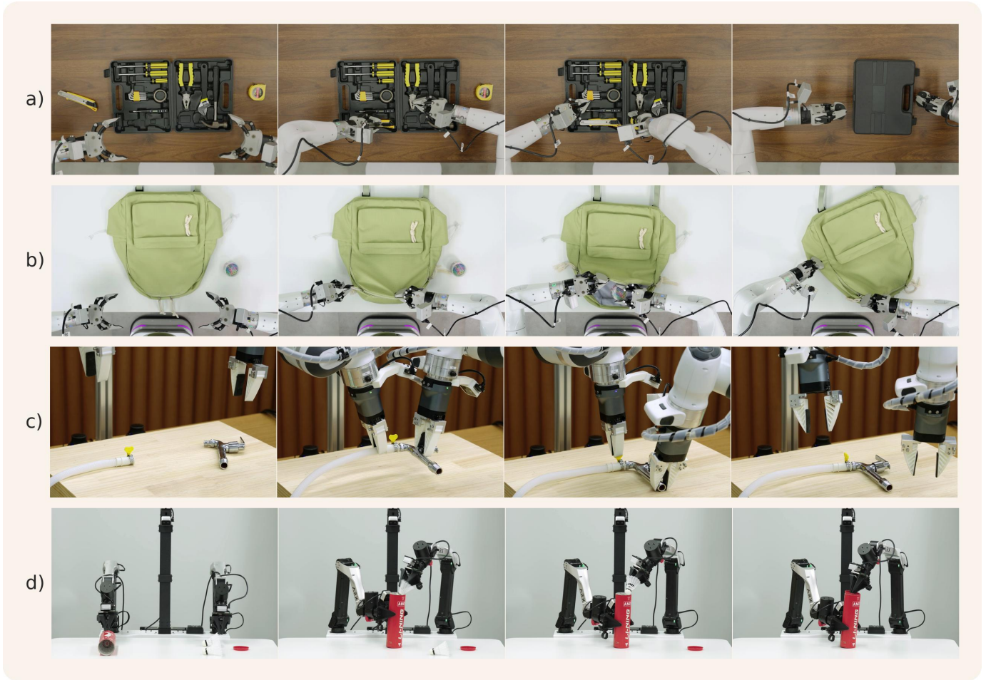
Fig. 3. Illustrations of our evaluation tasks. (a) Storing different tools on the desk into their corresponding places in the toolbox ( Toolbox ). (b) Unzipping the school bag, storing objects into it, and zipping up ( School Bag ). (c) Connecting the hose to the faucet and securing it ( Faucet ). (d) Storing the badminton shuttlecocks and closing the lid ( Badminton ).
